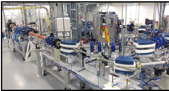
Figure 5. IR-THz FEL at Fritz Haber Institute (Berlin). Turn-key electron beamline was supplied by Advanced Energy Systems, Inc (AES). Wavelength region 0.004 – 0.4 mm [14]. Courtesy AES.
